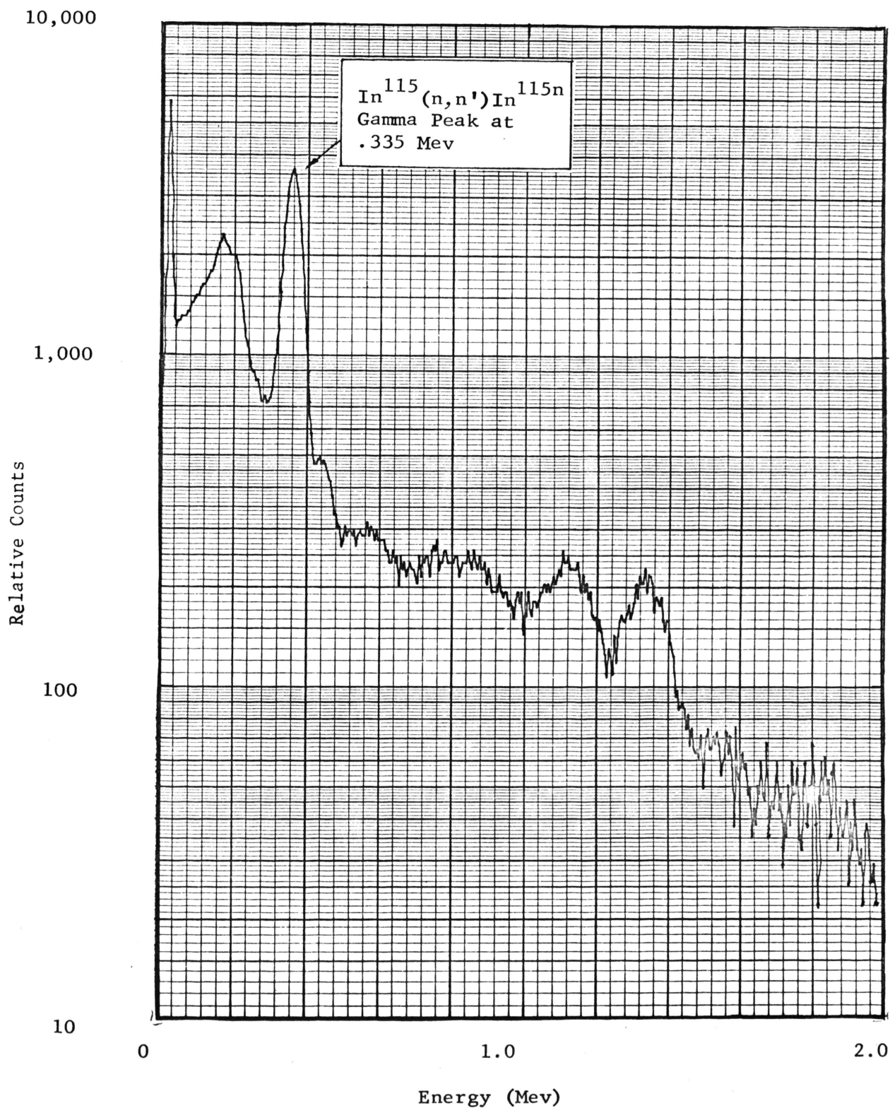
Figure B.6 Indium Gamma Spectrum 15.48 hours after Irradiation Relative Counts versus Energy
